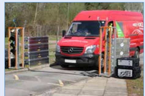
Deployed Configuration: Pop-up Vehicle Portal
